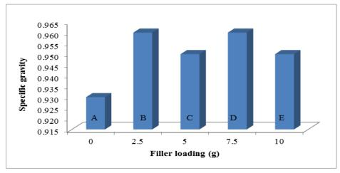
Figure 5: Specific gravity of natural rubber latex chitosan composites (A-E)
