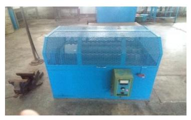
Figure 3: Ball mill machine
